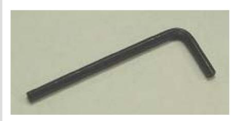
used to tighten or loosen the camera pedestal on top of MBC
