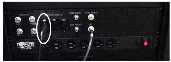
1. Turn on main power switch on rear panel of cabinet (red light means it is on.)
